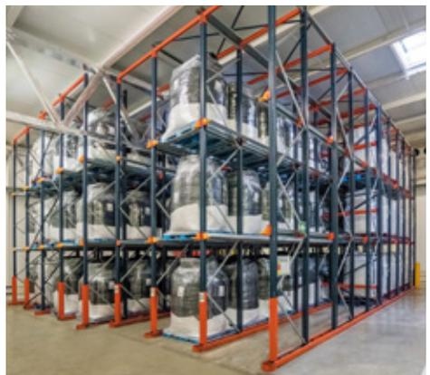
FUNCIONAM COM SISTEMA LIFO (*LAST IN, FIRST OUT*) OU FIFO
